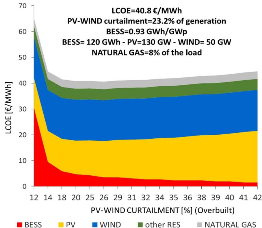
To reach least-cost production, an **optimal balancing** between solar and wind overbuild/curtailment and storage must be determined. A **small residual** use of **natural gas** could also be considered to further minimize costs and maximize flexibility.
