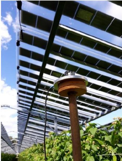
Figure 4. PAR sensor below solar panels
