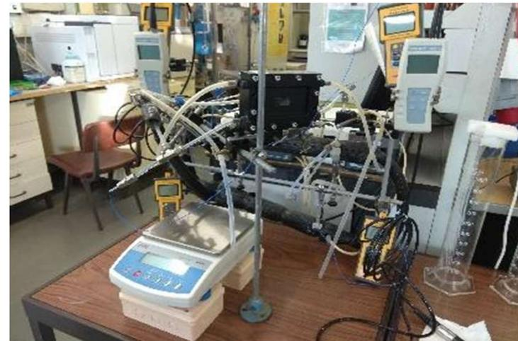
$\text{H}_2\text{SO}_4$  AS A STRIPPING SOLUTION IN THE PERMEATE
