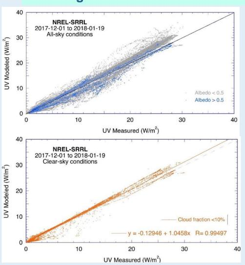
Modeled vs. measured 1-min UV global irradiance under all sky conditions at SRRL for low and high surface albedo conditions.
