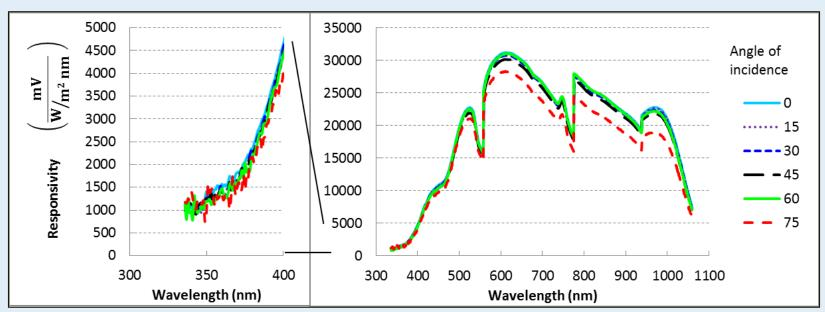
Responsivity compared to wavelength for various angles of incidence. The responsivity is nearly constant as the angle of incidence changes. Only when the angle of incidence is increased to 75° is there a noticeable change in the responsivity compared to the other angles. A detailed view of the wavelengths from 300–400 nm is shown in the left panel.
