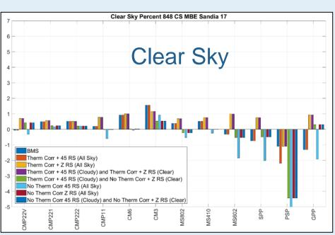
Newer radiometer designs have low cosine response and thermal offset and might not require correction.
